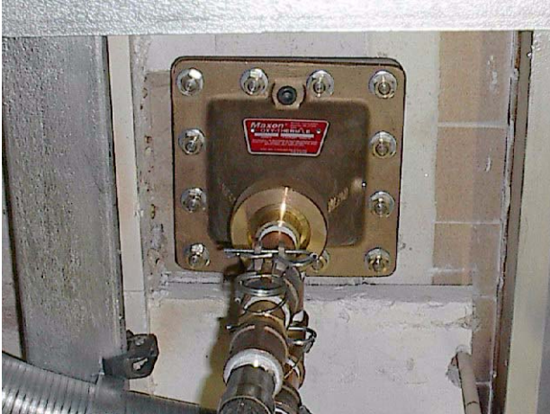
OXY-THERM® LE mounted on a glass furnace
